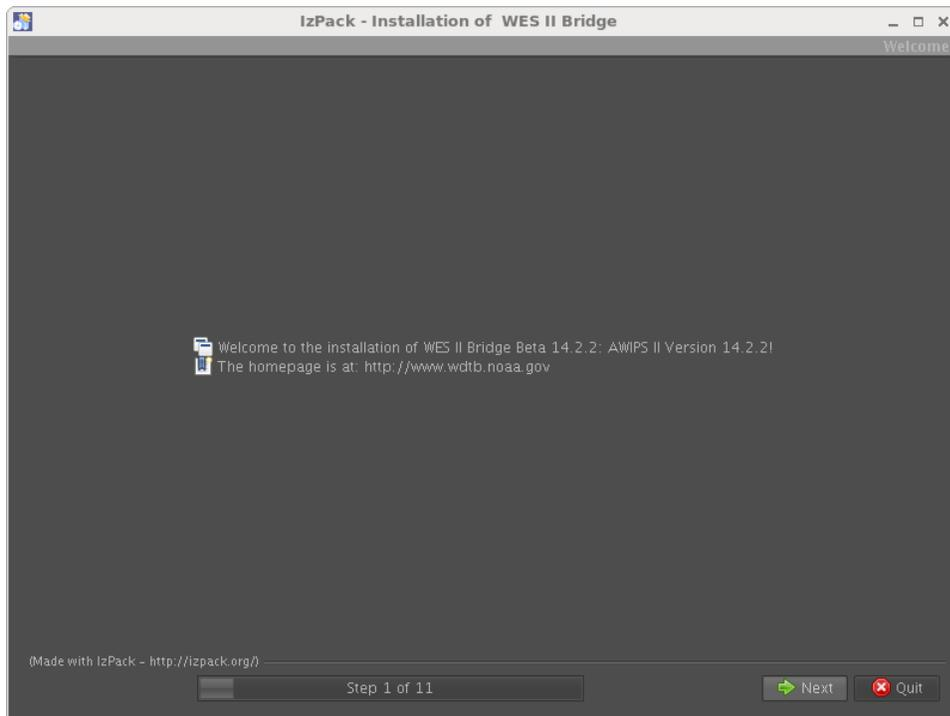
The WES-2 Bridge Installer not only installs the WES-2 Bridge software, but it also installs and configures the EDEX instances that are required for WES-2 Bridge to work. So you will run the installer either (1) when it's time to upgrade WES-2 Bridge, or (2) after you've upgraded the AWIPS-2 Build on the WES-2 Bridge machine in order to make EDEX instances that are compatible with the upgraded AWIPS-2.
