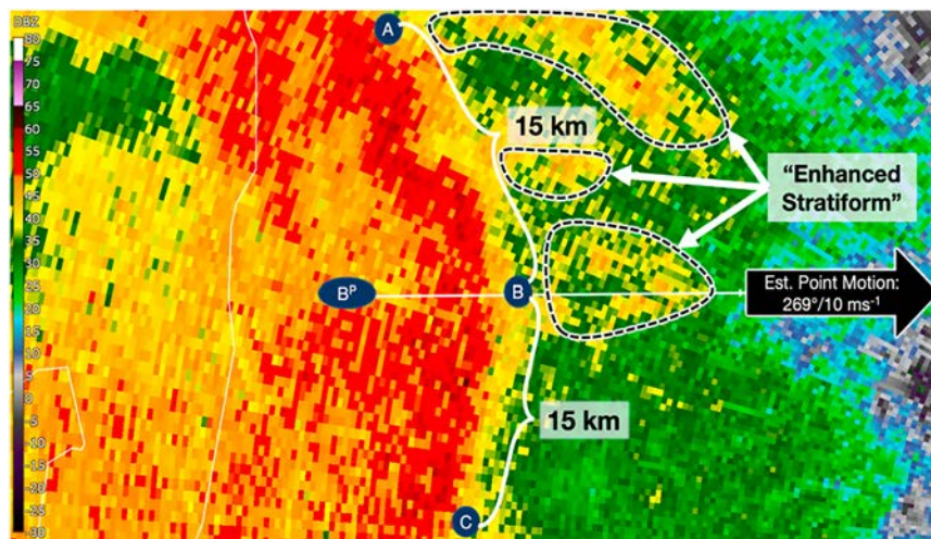
FIG. 9. A portion of a study QLCS across northern Michigan on 28 Aug 2018. Image from KAPX (at 0.5° elevation) valid at 2325 UTC. Point “B p ” represents position of point “B” (analysis point) at the prior analysis period (i.e., full volume scan), which is used to determine the storm motion vector and the path along which U-to-R distances are computed. Points “A” and “C” represent additional analysis points in the along-line direction at 15-km intervals.
