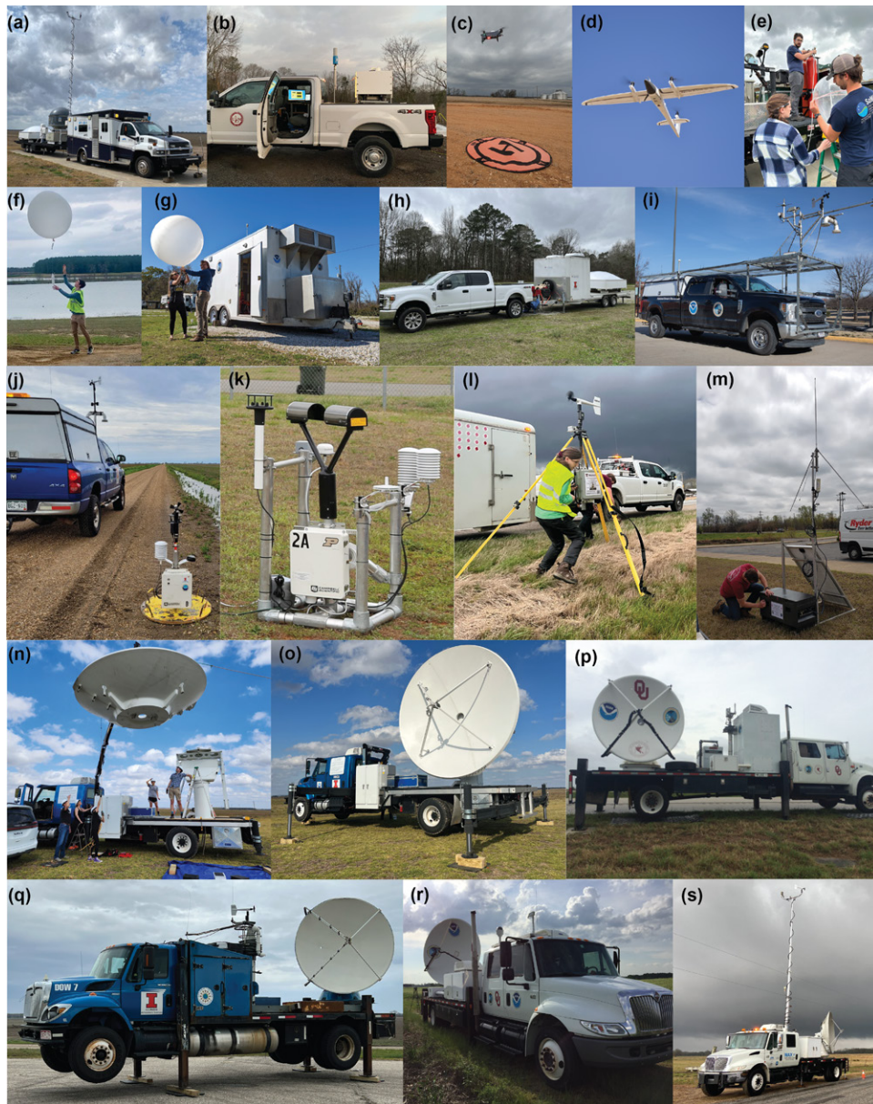
FIG. 1. Some of the instruments used during PERILS: (a) UAH MIPS, (b) ULM DWL, (c) OU CopterSonde, (d) NSSL/CIWRO UAS, (e) SBU preparing a SwarmSonde, (f) UIUC/NCSU sounding launch, (g) sounding being launched at the OU CLAMPS, (h) UIUC wind profiler, (i) NSSL MM, (j) UIUC MM and Pod, (k) Purdue PIPS, (l) TTU StickNet being set up, (m) NSSL LMA being set up, (n) UIUC COW radar being set up, (o) UIUC COW radar ready to operate, (p) OU SMART-R radar deployed, (q) UIUC DOW7 radar deployed, (r) NSSL NOXP radar deployed, and (s) UAH MAX radar deployed.
