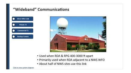
**Private T1:** This type of wideband link is used when the distance between the RDA and RPG is between 400 and 3000 feet. This configuration link occurs most commonly when the RDA is adjacent to the NWS Weather Forecast Office (WFO). Approximately half of the NWS WSR-88D site connections use this type of primary communications link.
