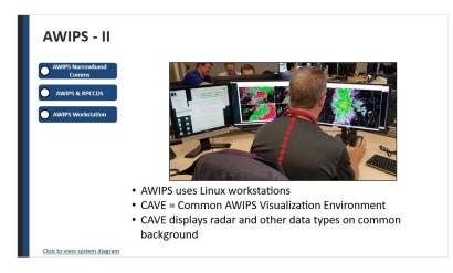
**AWIPS Workstation:** AWIPS uses Linux-based workstations to display the radar image products and alphanumeric data. The primary application used for radar data display and analysis is the Common AWIPS Visualization Environment (CAVE). CAVE can display:
