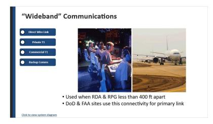
**Direct Wire Link:** Direct wire links connect the RDA and RPG when the distance between them is less than 400 feet. This WSR-88D configuration occurs most often when the RPG is located in the RDA shelter. All Department of Defense (DoD) and Federal Aviation Administration (FAA) sites use this type of connectivity for their primary link.
