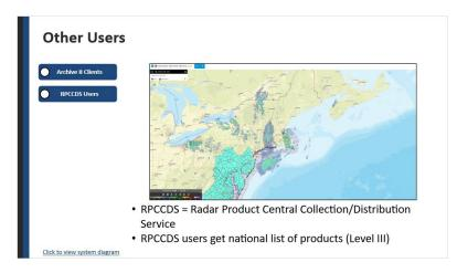
**RPCCDS Users:** Other users wanting to view WSR-88D products can access a predefined set of real-time products via the Radar Product Central Collection/Distribution Service (RPCCDS). The AWIPS data server sends these products through a dedicated connection to the Network Control Facility's servers at Silver Spring, MD. From there, the data can be accessed by users in real-time via: - The NWS Ridge web site,
