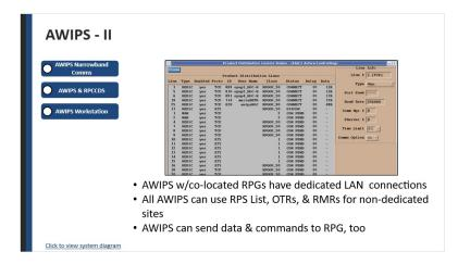
**AWIPS Narrowband Comms:** All AWIPS sites with co-located RPGs have a dedicated TCP/IP connection from the AWIPS LAN to the RPG LAN. For NWS sites with MSCF control of DoD or FAA radars, AWIPS connects to those RPGs by a Private IP connection. All AWIPS sites can also access data from non-dedicated RPGs using RPS Lists, as well as either the One-Time Request or Radar Multiple Request processes through the AWIPS WAN.
