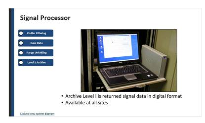
**Level 1:** The WSR-88D has the ability to record the original returned signal in a digital format (i.e., Archive Level I). Archive Level I recorders have been available at all RDAs since the fielding of RDA/RPG Build 19. The data recorder is a two terabyte removable drive.
