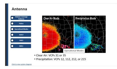
**Operational Modes:** In addition to VCPs, the WSR-88D has two operational modes which play a part in antenna positioning: Clear Air mode and Precipitation mode. The operational mode of the radar determines which VCPs are available to be used. For example:
