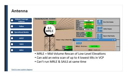
**MRLE:** The latest dynamic scanning feature added to the WSR-88D is the Mid-Volume Rescan of Low-Level Elevations (MRLE; Chrisman, 2016). During severe weather operations, MRLE can be used to collect an extra scan of up to the lowest four tilts in the volume scan. Like SAILS, these extra tilts are collected during the middle portion of the volume scan. MRLE and SAILS cannot be enabled concurrently, so you have to choose one option or the other.
