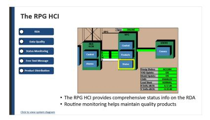
**Status Monitoring:** The RPG HCl offers comprehensive status information on the condition of the RDA, the RPG, and certain users. This information must be monitored frequently to ensure proper system operation so that all users continue to receive quality products.
