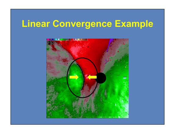
Here is a real-world example of a linear storm-scale convergence signature. In this case, a QLCS is approaching the RDA from the west, and a segment of the line is bowing out at this point, creating an enhanced convergence signature. Areas of enhanced convergence along a line segment could lead to mesovortex formation, which can enhance the wind threat and increase the probabilities of a tornado in areas of vorticity that are generated.
