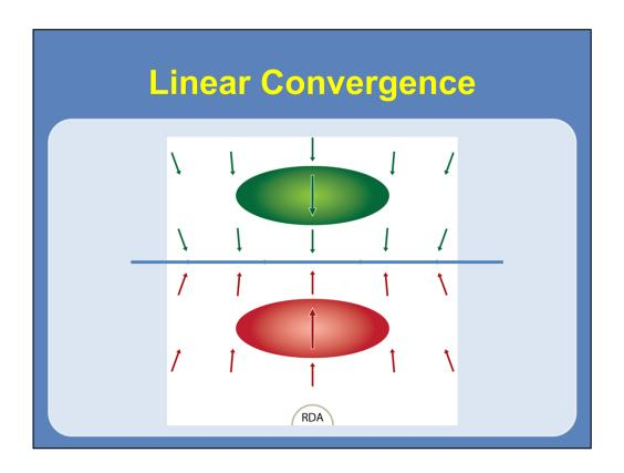
Here is a basic diagram of a convergent velocity signature focused along a linear feature. As you can see here, both the maxima still lie along the same radial with the outbound velocity maximum closest to the RDA. The exception is that these maxima are elongated across a number of radials at about the same range from the RDA.
