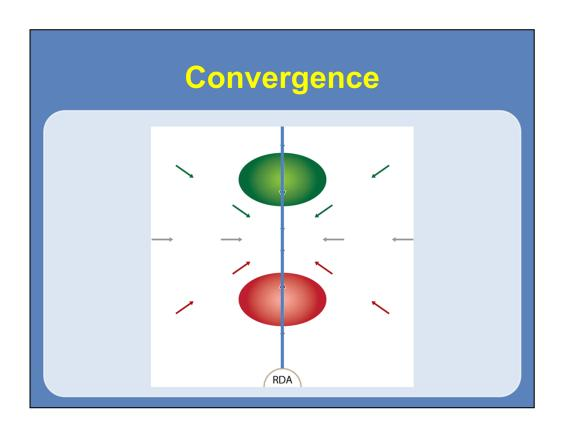
Here is a basic diagram of a convergent velocity signature. As you can see here, both the maxima lie along the same radial with the outbound velocity maximum closest to the RDA.
