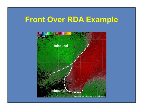
Now moving forward in time with the real-world example, the frontal boundary is now at the RDA. The inbound velocities are located to the south and west of the RDA ahead of the boundary and to the northwest of the RDA behind the boundary. A sharp change in speeds indicates the location of the boundary. Also note the backing wind profile ahead of the front.
