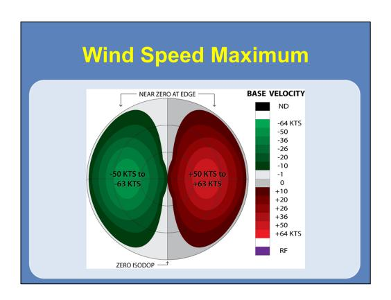
A wind speed maximum is identified by closed isodops surrounding a maximum velocity value. Here is a depiction of a low-level wind speed maximum, as if we had a low-level jet over weak surface flow and underneath a layer of near zero winds at the height that is represented by the farthest extent of the PPI. Starting near the RDA, you can see winds increase up to a closed area of 50-63 kts between the first and second range rings. From there, they decrease to near zero at the edge of the display.
