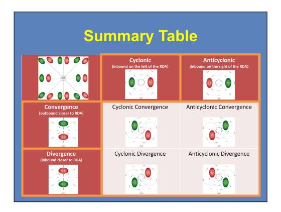
Let's go ahead and summarize storm-scale velocity signatures. Convergence signatures have the velocity maxima lie along the same radial with the outbound maximum closest to the radar. Divergence signatures have the velocity maxima lie along the same radial with the inbound maximum closest to the radar.
