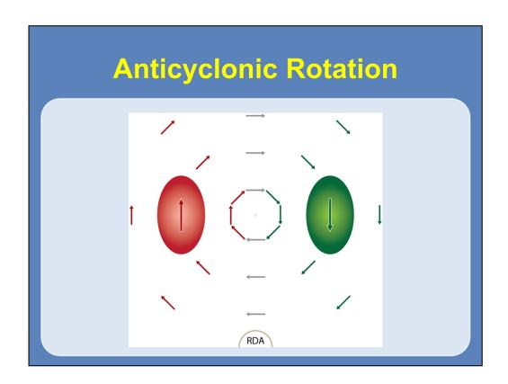
Now with the pure anticyclonic rotational signature, both velocity maxima are again equidistant from the radar with the inbound velocity maximum on the right side of the signature.
