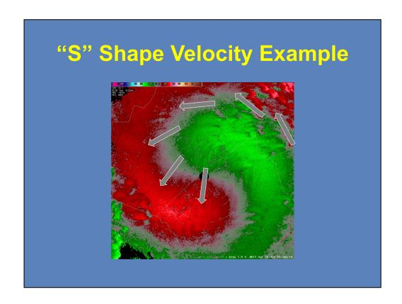
Here is a real-world example of veering winds with height. There is a "S" shape to the zero isodop, with winds from the north-northeast near the surface to winds from the south near the edge of the display. Thus, the winds are veering with height throughout the entire layer.
