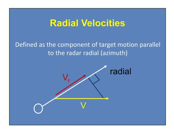
Before we begin to look at conceptual models of velocity patterns, we need to discuss radial velocities. A radial velocity is defined as the component of target motion parallel to the radar radial, or azimuth. In this diagram, you can see the actual target motion (yellow arrow) and the radial velocity target motion (red arrow) along the radial (white arrow).
