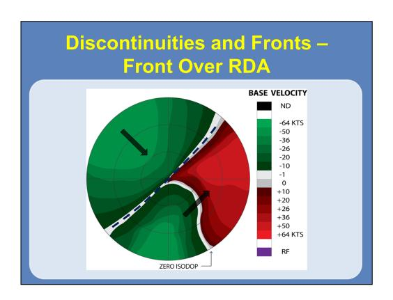
Moving forward in time, here is a graphical representation of a frontal boundary now located over the RDA. The boundary is still oriented from southwest to northeast, as seen by the zero isodop. The winds are from the northwest behind the boundary, while they are generally from the southwest in a veering pattern ahead of the front.
