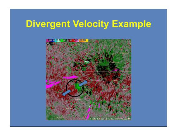
In this real-world example, there is a divergence signature located to the west-southwest of the RDA with a circular outflow pattern. This occurred just after a downburst from a thunderstorm. Note that the maximum inbound velocity is closer to the RDA than the maximum outbound velocity.
