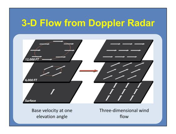
By using this concept, you can determine the wind flow at various levels and construct a three-dimensional wind profile of the atmosphere around the RDA. In this graphic here, you can see that with one elevation scan, the flow can be determined at different ranges, which are proportional to different heights. The flow at each range can then be assumed for a constant altitude.
