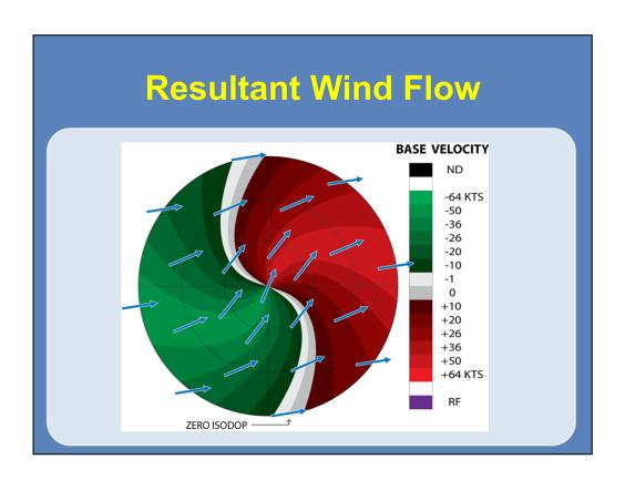
By using the methods described previously, we can determine the wind direction at any range (or height). It is important to draw the arrows perpendicular to the line from the RDA (radial), not the zero isodop itself.
