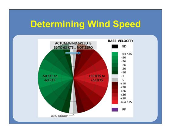
Now that we have seen how wind direction is determined, it is time to look at wind speed. Staying with the homogenous westerly flow example, we can easily tell the maximum wind speed from the radar either looking into or directly away from the wind. This example shows a constant wind speed with height of 50-63 kts. Even though the radial velocity is zero at the zero isodop, the actual velocity is still 50-63 kts.
