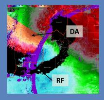
When interpreting velocity data, the radial velocities are displayed, which are not the true velocities. Also, the RPG dealiases velocities while the RDA performs range folding. These tasks are effective most of the time, but failures do occur, which can inhibit your ability to interpret velocity products.
