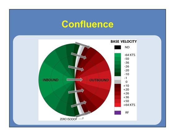
Looking at a diagram at what a confluent wind flow would be, you can see that the outbound velocities are now on the inside of the bow-shaped zero isodop. Here, the winds are coming together over the RDA.
