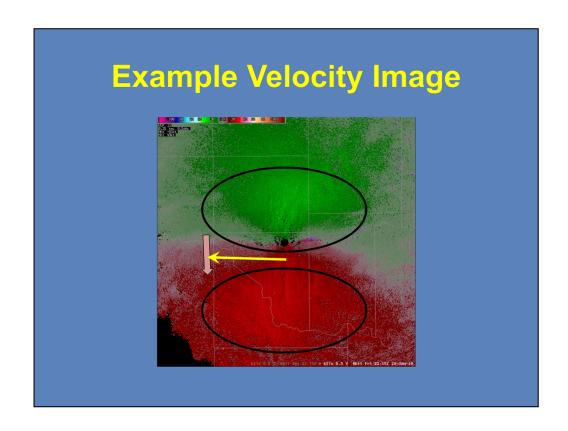
Here is a velocity example that represent some of the concepts learned in the previous slides. First, you can see a fairly straight zero isodop extend from east to west across the display. With the inbound velocities north of the RDA, the general flow is from north to south. You can also see that the wind speed maximum is close to the radar. As you move farther away from the radar in the N-S direction, the maximum velocity values decrease, signifying a low-level wind maximum.
