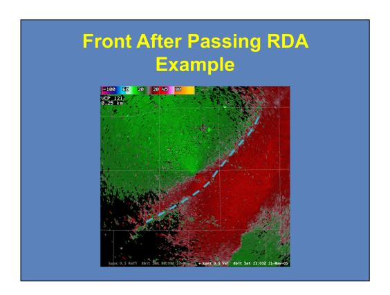
Back to the real world example, the front is now located to the southeast of the RDA, which is denoted by the blue line here. Notice that this front is losing definition with time. Only to the southwest of the RDA is there a leading edge of inbound velocities. Otherwise, use the leading edge of the enhanced outbounds as the frontal interface.
