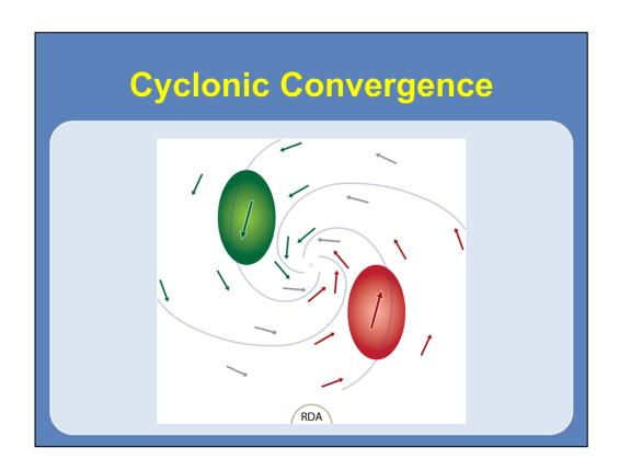
Now to make things more complicated, we will show combinations of both rotation and convergence or divergence. This is an example of cyclonic convergence. First note that both the maxima are not on the same radial and not equidistant from the radar. Here, the outbound maximum is closest to the RDA, signifying convergence, and the inbound maximum is to the left, signifying cyclonic rotation.
