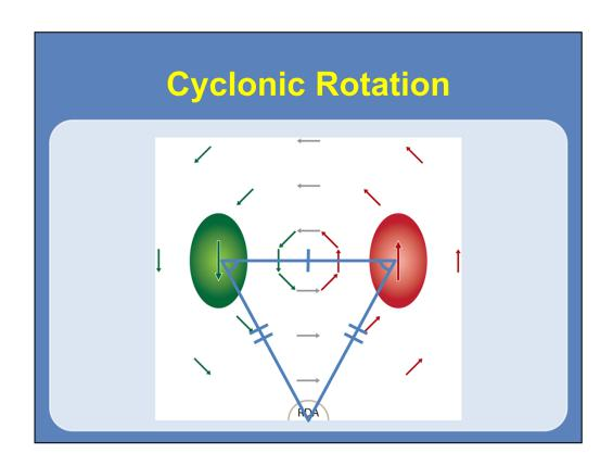
Here is a basic example of a pure cyclonic rotational signature. As you can see here, both of the velocity maxima are equidistant from the RDA with the maximum inbound velocities on the left side of the signature.
