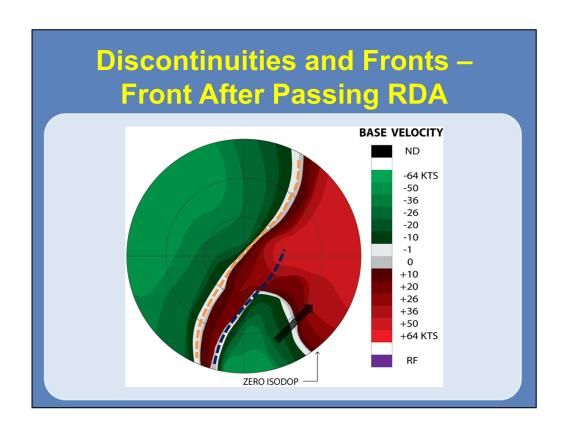
The front has now passed over the RDA and is now located to its southeast. The winds ahead of the front (southeastern 1/3 of the display) are still from the southwest. The front is approximately located where the blue line is drawn. Behind the front, the winds are now backing with height.
