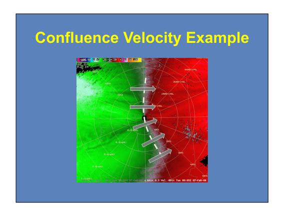
Here is a real-life example of a confluence zone as seen by the WSR-88D. A lake effect snow band is passing over this radar from southwest to northeast. You can see that the zero isodop bends in a way that the outbound velocities are on the inside of the bowing shape.
