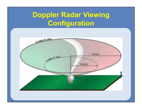
When you are looking at a velocity product, you are viewing the display from above looking into a cone. As you move farther away from the RDA, you are also increasing in height above the ground.
