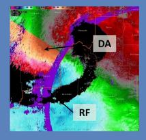
Just like Lesson 1, we will recall that when interpreting velocity data, the radial velocities are displayed, which are not the true velocities. Also, the RPG dealiases velocities while the RDA performs range folding. These tasks are effective most of the time, but failures do occur, which can inhibit your ability to interpret velocity products.
