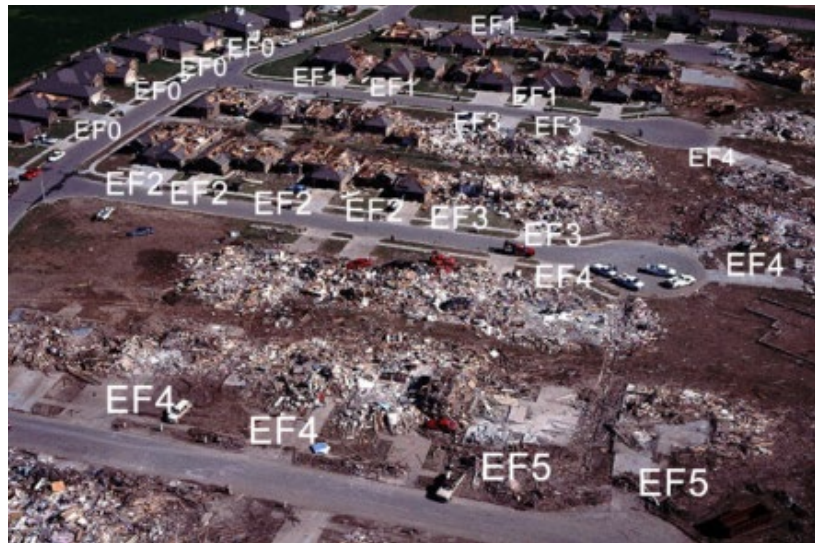
Gradations of damage ranging from EF0 (in upper-left corner) to EF5 (in lower-right corner). EF-scale ratings have been assigned to select one- and two-family houses.
