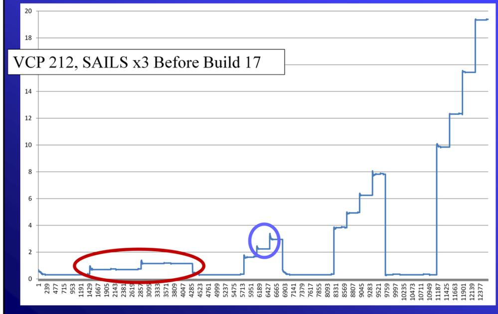
Here is a similar example for VCP 212, with SAILS x3, before the installation of Build 17. You can see the three times that the antenna drops down to collect the SAILS cut data. The purple circle shows us the most obvious wobble at the beginning of an elevation, and this exists throughout the volume scan. There is also dithering highlighted by the red oval for the two elevation where it's easiest to see.
