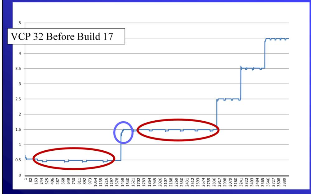
Here's an example from one of the Build 17 Beta sites. Before the installation of Build 17, this graphic shows you the antenna position for VCP 32. The purple circle shows us one of the transitions to a new elevation, which has some "bumps" in it. The red ovals show what is called "dithering" as the data are being collected. Dithering is occurring on all of the elevations.
