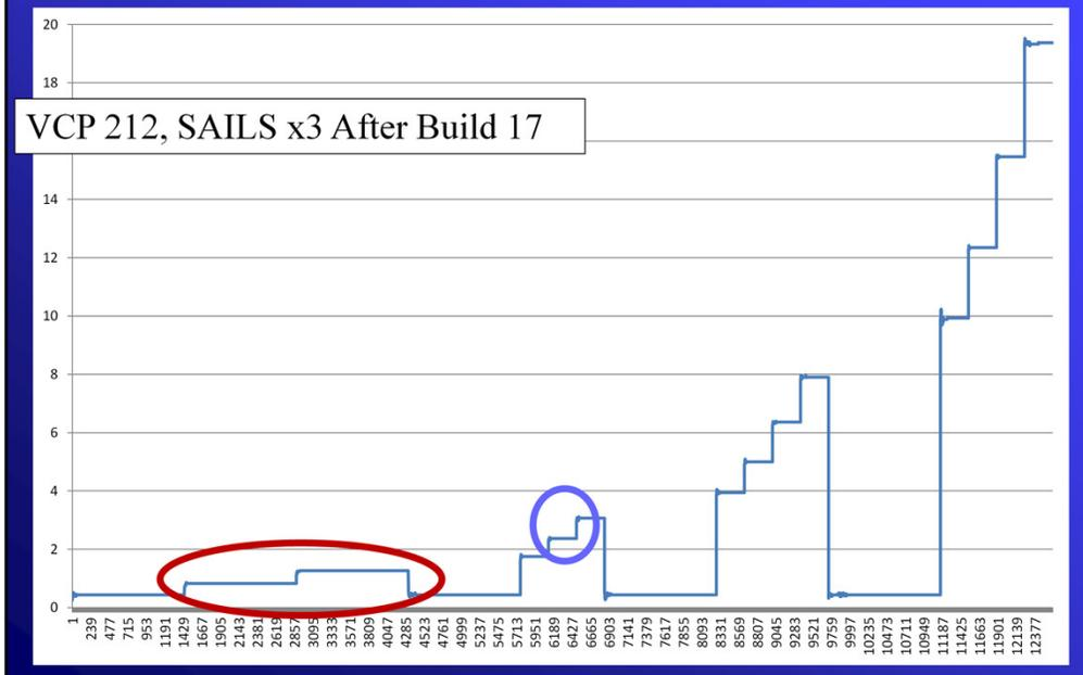
And now for VCP 212 after the installation of Build 17. Just as with VCP 32, there is much less wobbling when moving to a new elevation, and the antenna is much more stable while the data at an elevation are collected.
