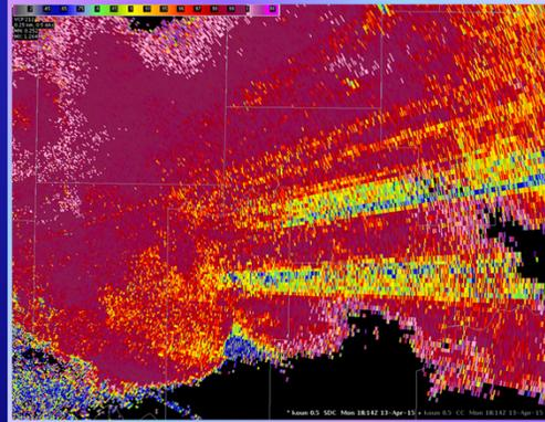
The Level II CC Product viewable in AWIPS is identified as the Raw CC (SDC). It will be available with AWIPS-2 Operational Build 16.1.1. You may notice a menu entry for “Raw PhiDP (SDP)” just below it. That will become available with RDA/RPG Build 17.0, with the deployment currently scheduled to begin during the Fall of 2016 and there will definitely be training on that product!
